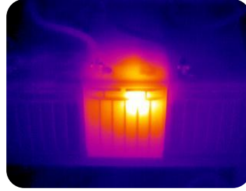
Infrared image of overheated battery Photo source: Predictive Service
